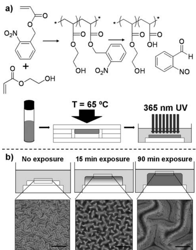
Fig. 1 Schematic of gel formation and light exposure. (a) Thermal polymerization of HEA and 2-NBA is followed by irradiation with 365 nm UV light in DMSO to cleave 2-nitrobenzyl groups, leaving behind poly (HEA-co-AA). The crosslinking is not shown in the structure. (b) Polymer swelling in PBS is dependent on UV exposure and causes stress-induced wrinkling patterns on the gel surface. The wrinkle morphology is dependent on the time of light exposure. All scale bars = 100 \mu m.
